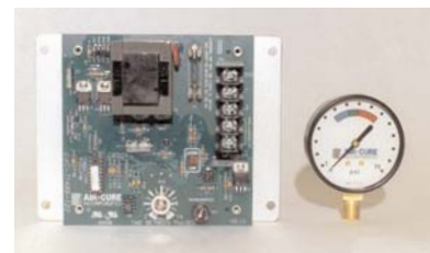
(right) New AC digital microprocessor timer controls the pulse cycle for cleaning air system with new pressure gauge.
