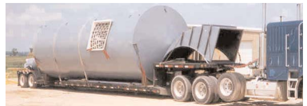
All-welded filter loaded on double drop trailer with bolt-on inlet scroll.
